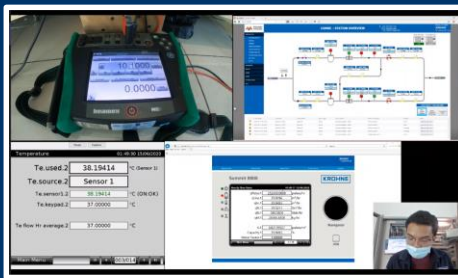
Pegaga new metering system - virtual FAT hosted via Microsoft Teams by Krohne from testing facility in Semeniyh.
