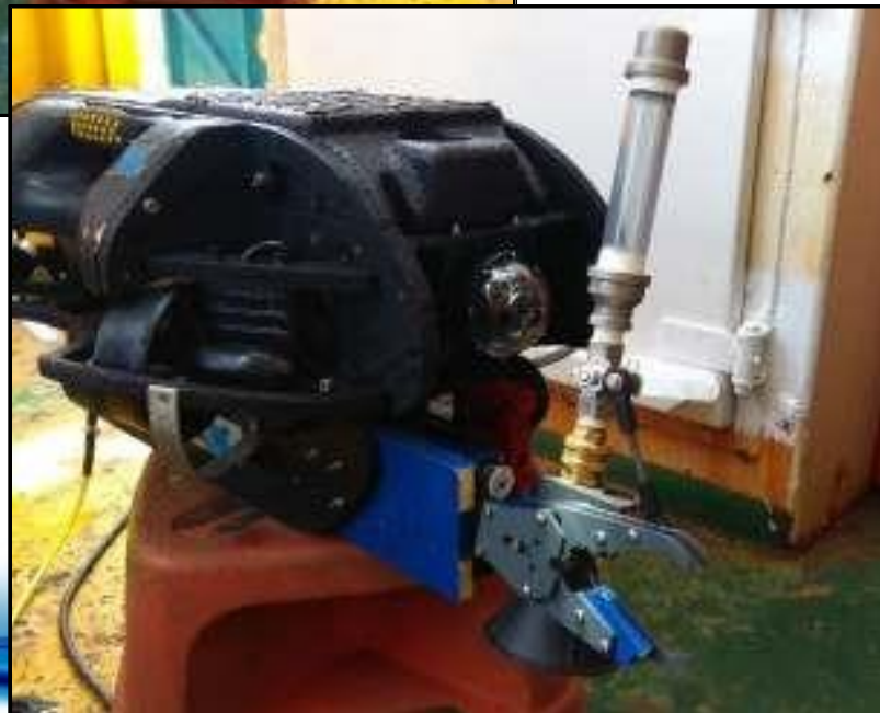
High-spec Mini-ROV ready for subsea gas sample retrieval
