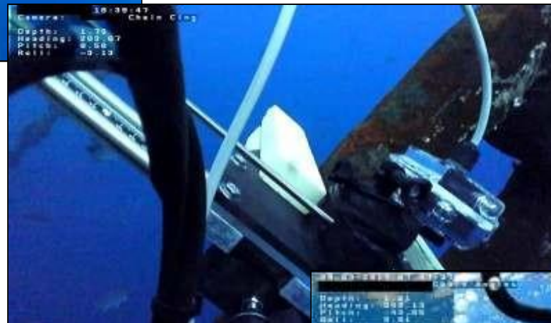
Mini-ROV mounted Calipers for Thickness Measurements (ABS approved)
