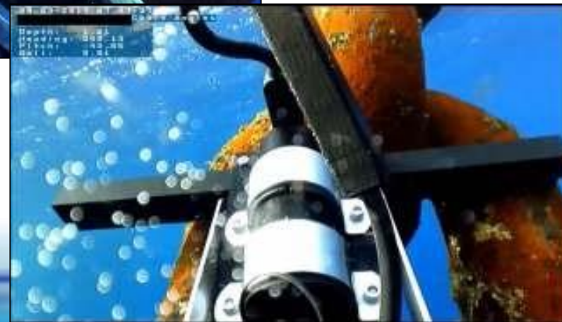
Chain incline Angle Measurements
