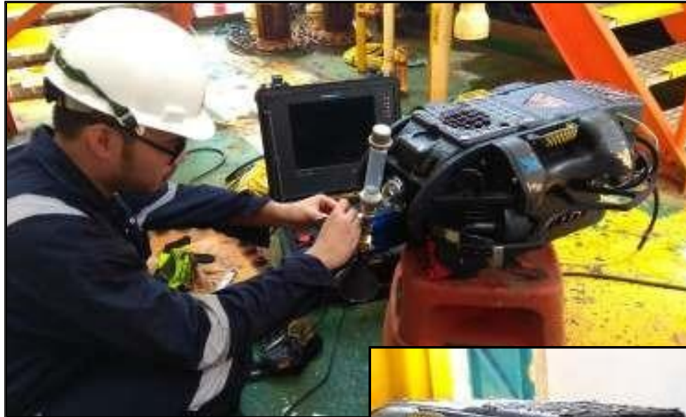
High-spec Mini-ROV rigged for Gas or Water sampling
