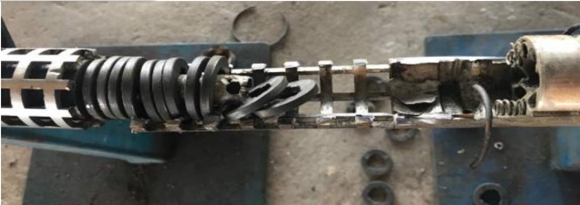
Sections of base pipe fully eroded away
