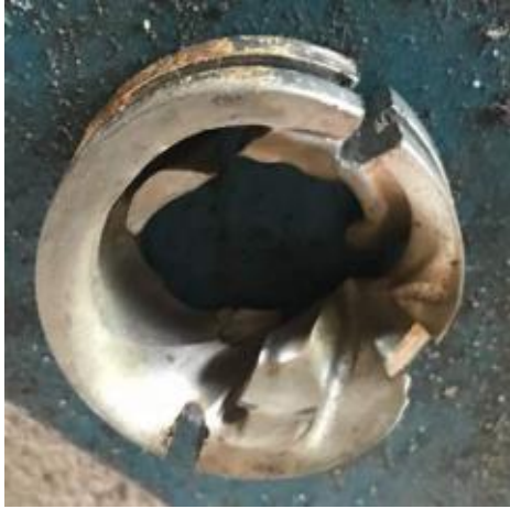
Metal seal ring badly eroded
