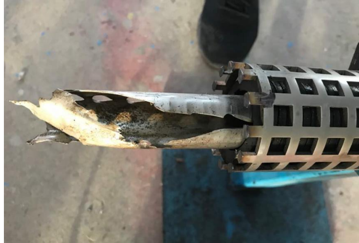
Base pipe almost fully eroded
