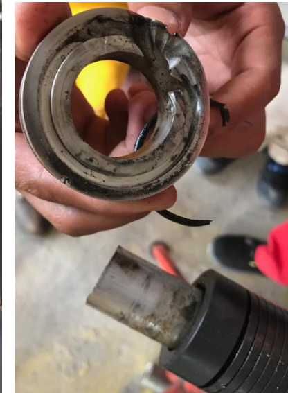
Metal seal ring badly eroded
