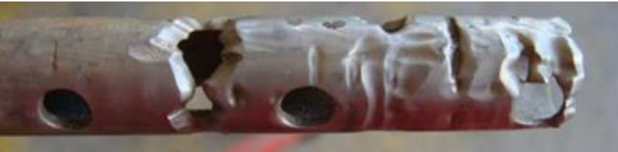
Sections of base pipe fully eroded away
